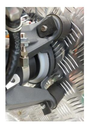
Put on the crankcase the two small rubber pieces given with the engine, to protect the crankcase from scratches
