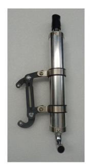
Insert the collars in the silencer and connect them to the exhaust flanges already assembled. Use 2 low flanged nuts M8x1,25
