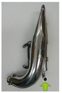
Assemble the silencer to the exhaust, with the spout of the silencer that points out
