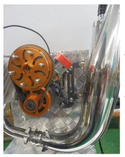
Now the exhaust is attached to the engine, but not yet completely fixed
