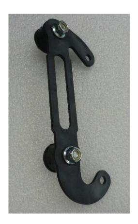
Connect the rubber mounts to the exhaust flange with 2 flanged nuts M8x1,25
