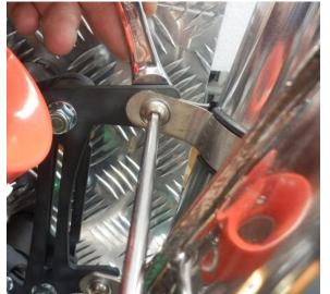
Now tighten completely the nuts of the collars, after you have found the right position of the collars on the silencer
