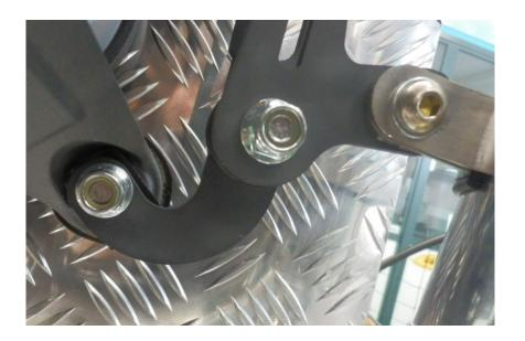
Insert the flanges of the exhaust in their seat. We recommend to use autofixing bolts
