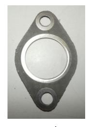
Prepare the exhaust gasket with the spacers of 0,3 mm on the small holes
