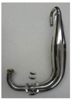
At this stage check that the manifold and the exhaust are aligned in the proper way
