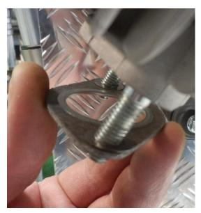
Put the gasket on the cylinder with the spacers on this side, then connect the manifold using a washer, a grower and an autofixing bolt
