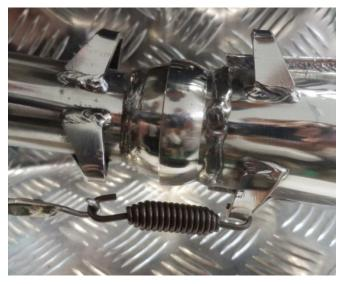
Fix the 3 springs one after the other. You could put some copper grease between the manifold sphere and the exhaust to avoid friction. Remember to put grease again every some hours of flight
