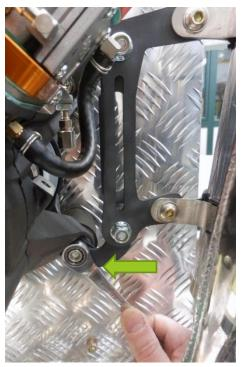
Tighten the lower bolt...
